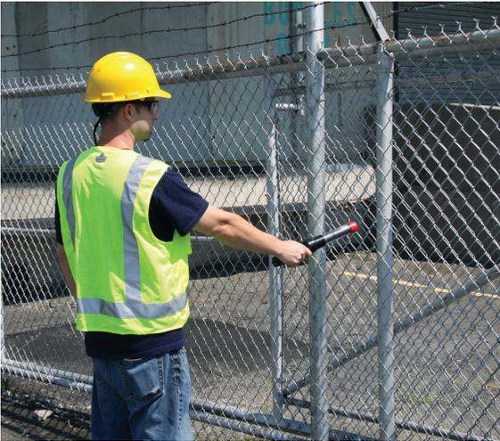
By testing fences and other objects for stray voltage, Seattle City Light has eliminated hazards.
