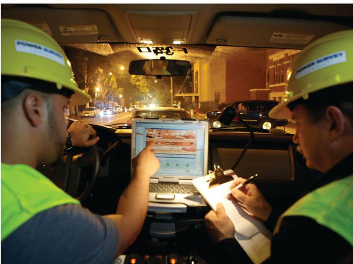
A Power Survey crew operates the SVD-2000 to detect electric fields from energized objects.
